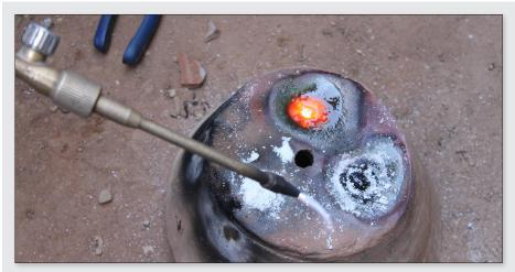
Figure 4. Gold has been concentrated and smelted to a small bead.
