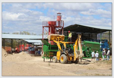
Figure 7. Mercury Recovery Plant (MRP) being loaded by tailings (Nicaragua).
