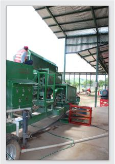
Figure 8. Mercury Recovery Plant (MRP) hooked up with Peter Plates (Nicaragua).
