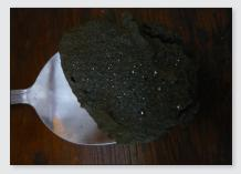
Figure 5. Mercury flour (droplets) in a spoonful of tailings (Philippines).
