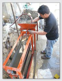
Figure 6. Prototype of "Peter Plates" in action (Philippines). Tailing slurry from the tub is passed over the plates in succession.
