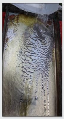
Figure 9. Large amount of mercury captured on Peter Plate (Nicaragua). The plate is about 20 cm wide.
