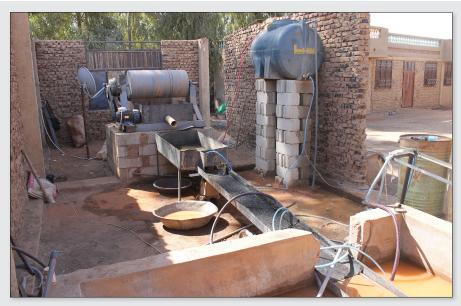
**Figure 1.** Efficient artisanal processing plant (Sudan) with mill and gravitational processing of pulverised gold ore. The ore is milled in the drum in the background, after which the fine-grained ore is passed through a system of sluices, which concentrates the heavy minerals, including gold.
