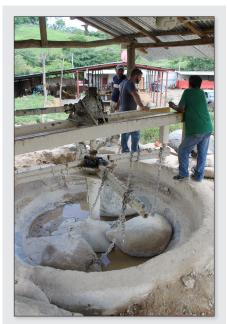
Figure 2. Low tech milling (rastra) with mercury addition (Nicaragua). The boulders mill around slowly for a couple of hours. When milling is complete, the cavity is cleaned of milled ore and mercury amalgamated with gold. The flour floats away.
