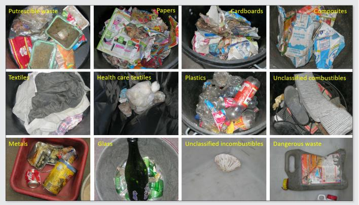
Figure 4. Example of coarse elements (>100mm) after sorting.
