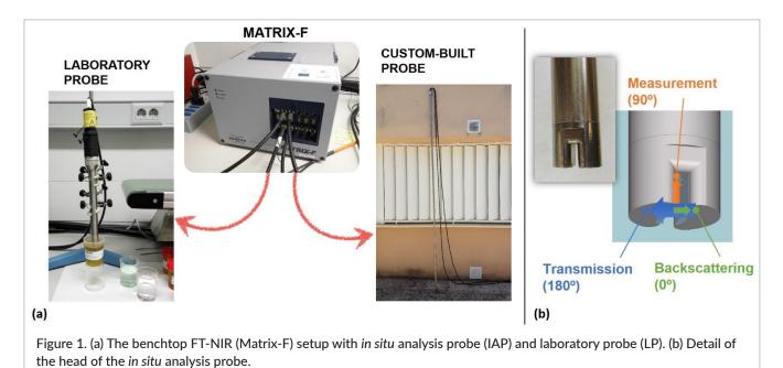
samples (Figure 1a). This equipment supports multiple modes of analysis and features six channels to connect fiber optic sensors.
