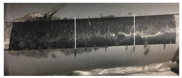
Figure 9. Defaced motorcycle fork painted with India ink (white lines demarcate the sections individually imaged and analysed).
