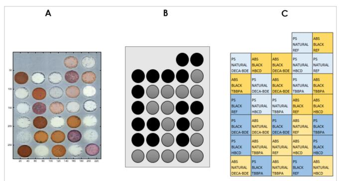
Figure 1. Calibration and test set of plastics for this study. A) False colour image of the plastics. B) Calibration (black) and Validation (grey) samples of plastics. C) Description of the plastic samples, type of plastics, version of these plastics (Natural or Black) and type of flame retardants.
