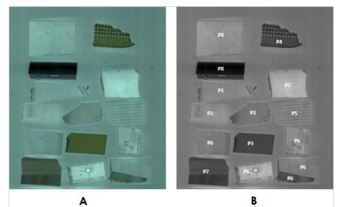
Figure 2. A) False colour image of the real samples of plastics. B). Composition of the real samples of plastics: P1 (ABS-Black-HBCD), P2 (ABS-Black-REF), P3 (ABS-Natural-HBCD), P4 (ABS-Natural-REF), P5 (PS-Black-Deca-BDE), P6 (PS-Black-TBBPA), P7 (PS-Natural-REF) and P8 (PS-Natural-TBBPA).
