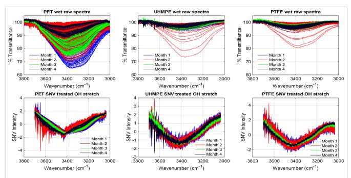
Figure 3. Effect of SNV normalisation on the OH  $\bar{v}_s$  region for PET (left), UHMPE (centre) and PTFE (right) along the time. The top portion of the figure shows the untreated spectra, whereas the bottom portion shows the effect of the pre-treatment.
