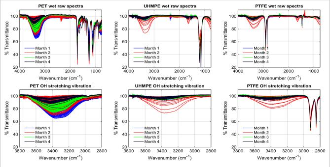
Figure 2. Raw (untreated) spectra of bulk polymers at all time points. Lower section focusses on the OH  $\bar{v}_s$  region of wet spectra. Intense spectral variation is seen for Mylar (PET)—Month 1.
