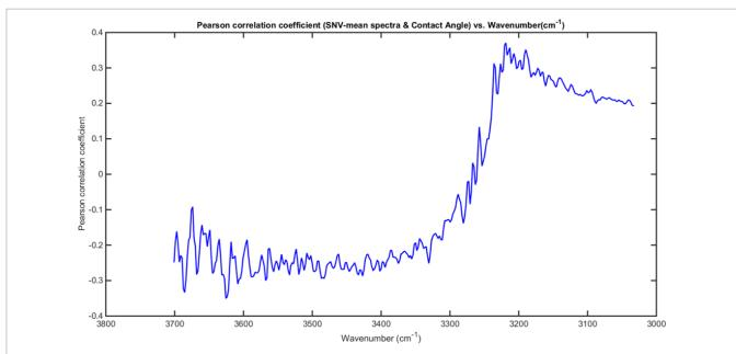
Figure 10. Pearson correlation coefficient calculated between SNV-mean spectra and CA data as a function of wave-number (cm<sup>-1</sup>). Very low correlation observed near 3200 cm<sup>-1</sup>(0.35).
