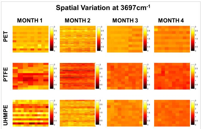
Figure 6. Spatial variation of % of transmittance intensity at 3697 cm<sup>-1</sup> for PET (top), PTFE (centre) and UHMPE (bottom). A lighter pixel colour indicates higher % of transmittance intensity of the wavenumber 3697 cm<sup>-1</sup> inferring lower hydrophobicity.
