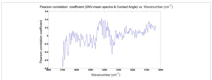
Figure 4. Pearson correlation coefficient between the intensity of the SNV-treated mean spectra of each wavenumber of the stretching vibration and CA data of each polymer. The wavenumber at 3697 cm<sup>-1</sup> shows a relatively high correlation coefficient (–0.76).
