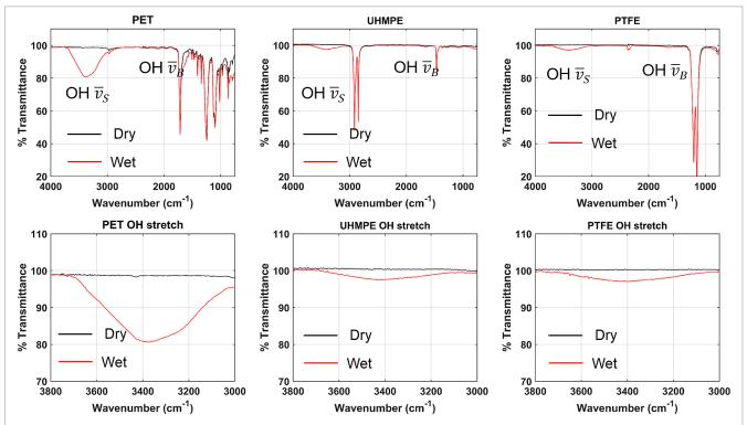
Figure 1. Raw dry (black line) and wet (red line) mean spectra from bulk polymers collected from the first month. Lower section focusses on the OH  $\overline{v}_s$  region which is free from overlapping native polymer bands.
