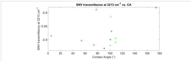
Figure 11. SNV transmittance at 3213 cm<sup>-1</sup> as a function of CA data for HMDSO-coated Si wafers (red—hydrophilic, green—hydrophobic, blue—superhydrophobic).
