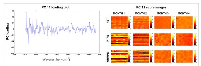
Figure 8. Loading plot for PC 11 (left) and spatial variation across PC 11 score images (right) for PET (top), PTFE (centre) and UHMPE (bottom) over time. Lighter colour of the pixel indicates higher intensity of the PC 11 loading prominent feature at wavenumber 3690 cm<sup>-1</sup> inferring lower hydrophobicity for PET and UHMPE.
