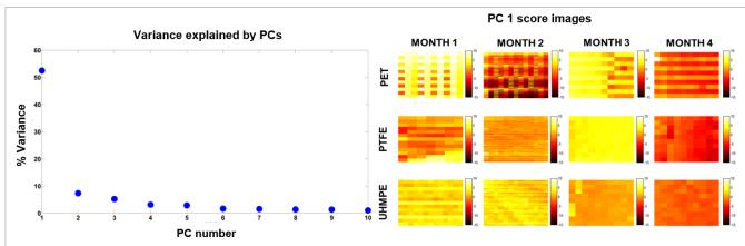
Figure 7. Variance explained by each PC (left). PC 1 accounts for almost 50% of the variation. Score images for PC 1 are shown in the right, where a lighter pixel colour indicates higher intensity of the PC score.
