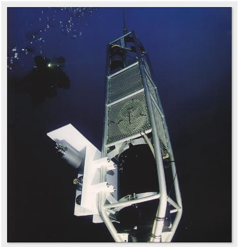
Figure 5. Fully calibrated bivalves are located in Biota Guard's subsea station (upper cage). The station shown here was deployed in a fjord in the Norwegian North Sea during one of Biota Guards full-scale testing campaigns. Credit: Vidar Skålevik.
