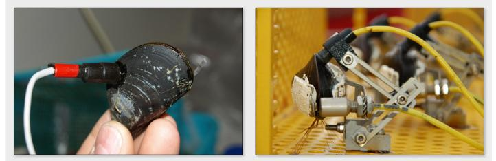
Figure 3. Instrumented bivalves fitted with an infrared sensor for heart rate determination (left), and with added calipers for recording valve gape (openingclosing) characteristics as well (right).
