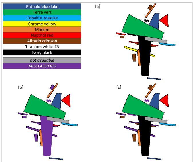
Figure 8. Graphical illustration of the bespoke painting ground truth with colour coding of paints (a) and classification results for Firefly IR Imager (b) and Red Eye 1.7 Imager (c).
