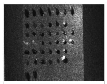
Figure 2. Single band image (at 3200 nm) of the test paint grid illustrating spatial intensity variation of collected reflected illumination.
